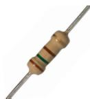
If we needed a 1K (or 1 kilo-ohm) resistor we would need a Brown, Black, Red combination (1, 0, +2 zeros). If we needed a 570K resistor the colours would be Green, Violet and Yellow.
